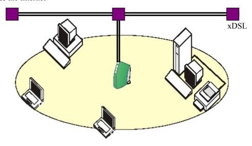
Figure 1-2 Connect to a Residential Gateway (RG)
